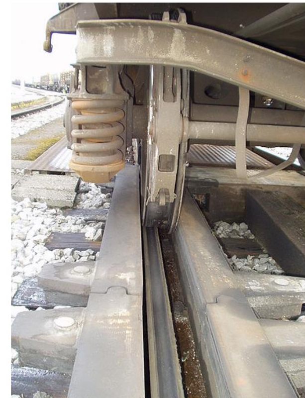
Mechanical and electro-dynamic retarders in shunting yards
