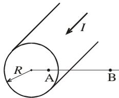
4. Determine the force on the unit of length acting on the conductors of two-conductors-line, the current  $i(t) = I_m \sin \omega t$  flows through the conductors. Draw the time function of the force  $F(t)$ , draw the direction of the force and calculate the maximal value of the force  $F_{\max}$ .
